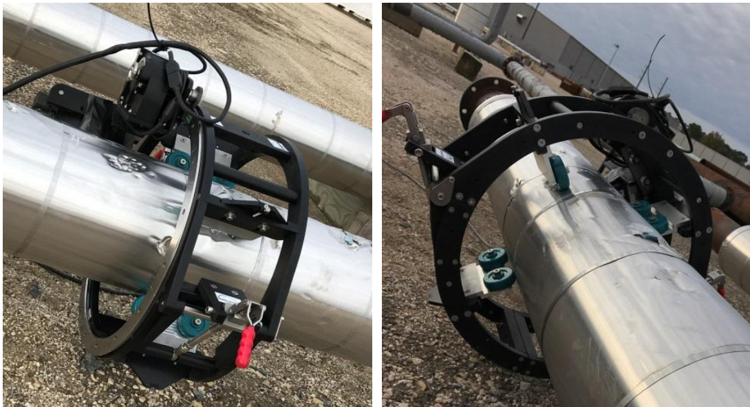
Figure 7: The semi-automatic scanning ring
