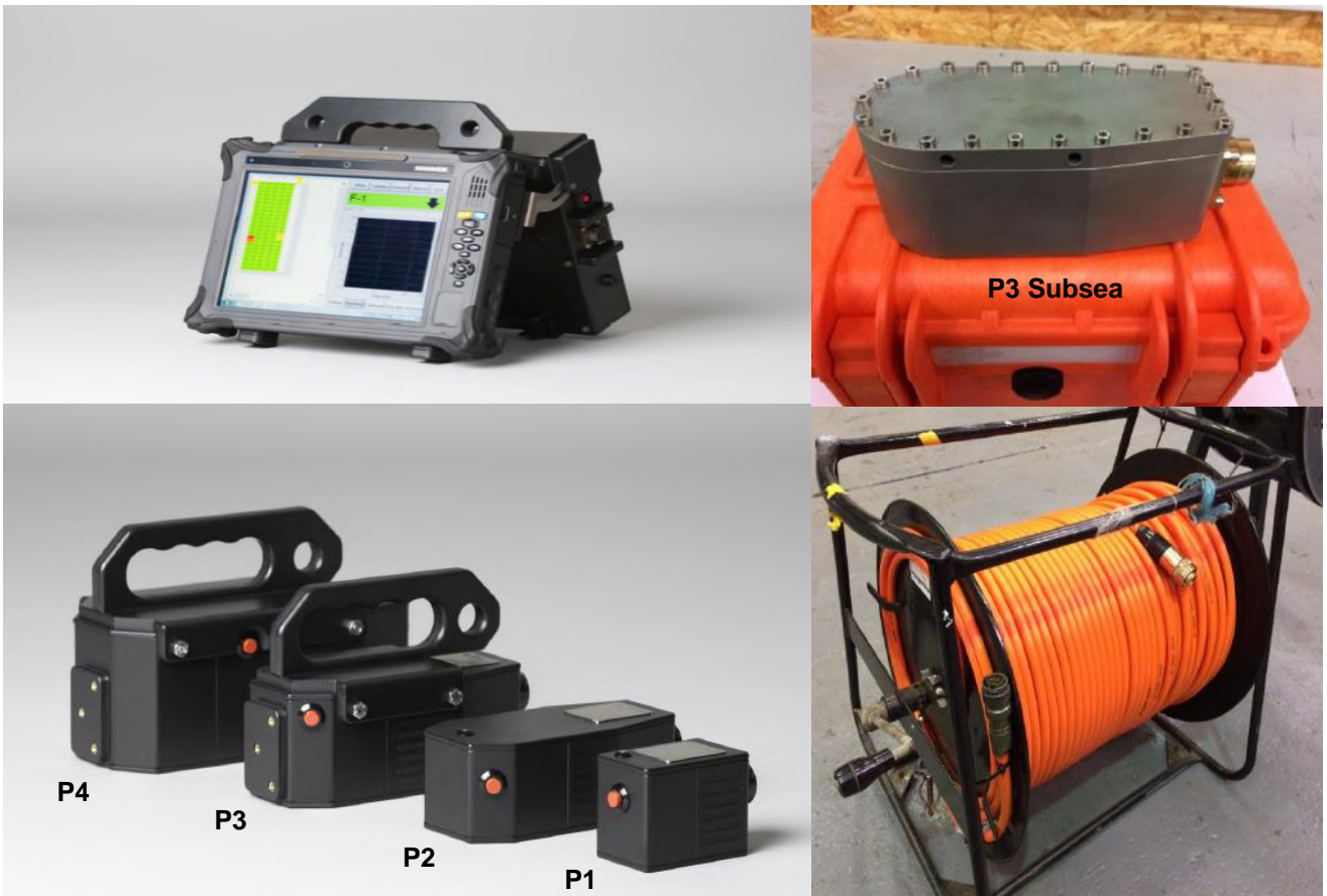
Figure 5: The PECT probes and equipment
