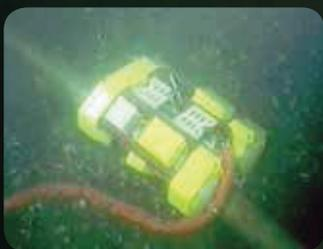
Feature: MEC-Crawler scanning the bend of the flexible pipe on seabed
