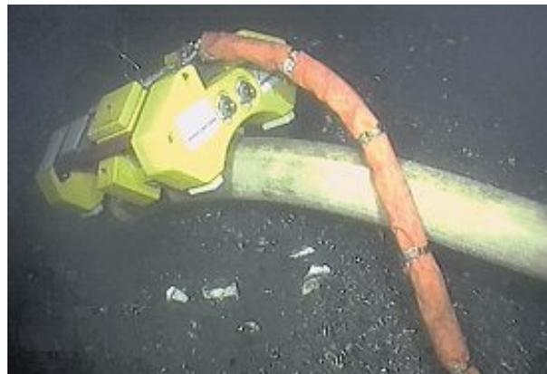
**MEC-Combi PipeCrawler (v2) inspecting a flexible pipe on seabed**
