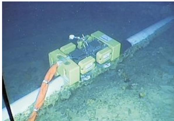
**MEC-Combi PipeCrawler (v1) inspecting a subsea pipeline**
