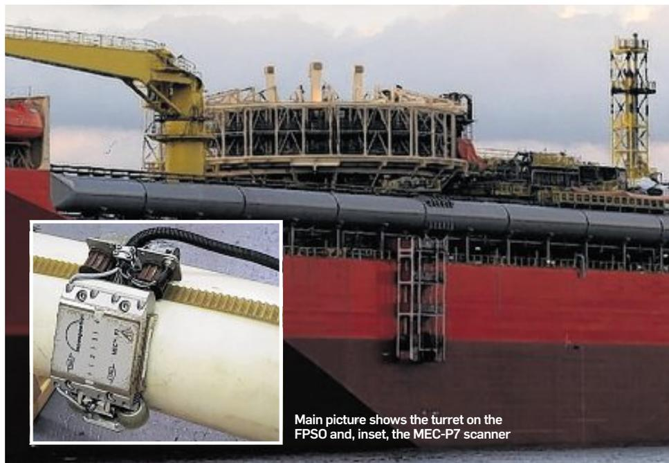
Main picture shows the turret on the FPSO and, inset, the MEC-P7 scanner
