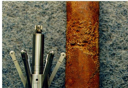
External corrosion near the lower bend
