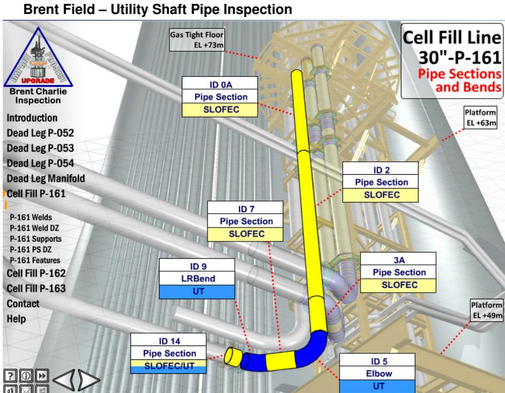
The pipe section was the subject of a SLOFEC™ scan by Innospection Ltd. However prior to the mobilization, a number of manual Ultrasonic spot checks with a 0° compression wave probe were showing some severe localized defects with diameter of 10-15mm and minimum remain wall of down to 2.6mm.
