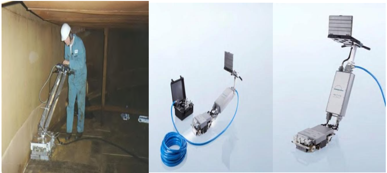
Figure 3: SLOFEC™ FS300 Floorscanner inspecting annular zone area next to the Tank wall; MEC-F15 Floorscanner – next generation and a further development of the SLOFEC™ Floorscanners
